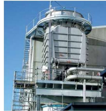
This vertical patented design is well suited to sludge thickening in industrial WWTPs, where the efficiency/surface ratio is strategic in investment choice
